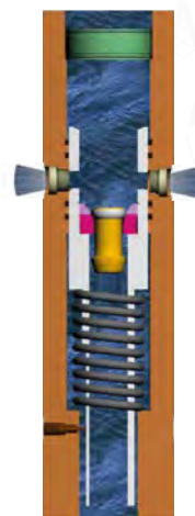
3. Open Position Flow thru Dart & Ports
