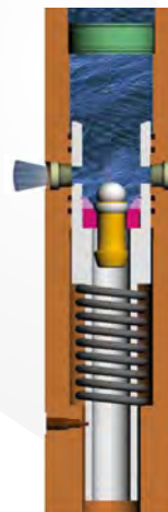
6. Open Position Flow thru Ports Only
