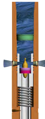
2. Open Position Flow through Ports
